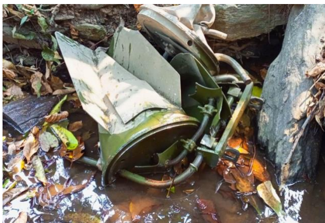
Cluster bomb remnants in Mindat after an April 2023 attack, with portions of the internal frame for holding submunitions still attached. © Chin Defence Force – Mindat , 14 April 2023
